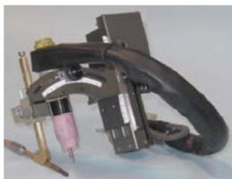
TIG / GTAW "standard" torch module
