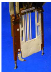
Hot wire, "narrow groove" torch module
